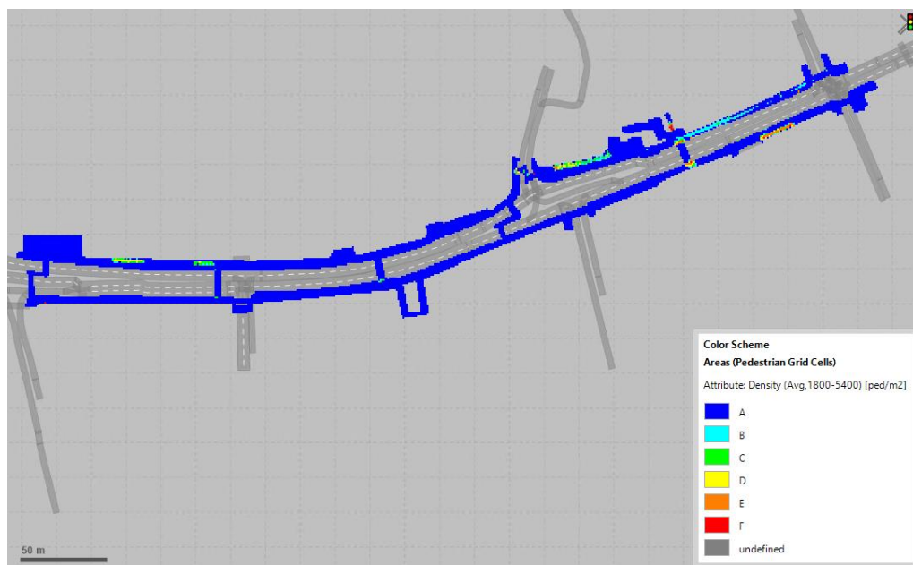
Figure 32 Example of evaluation of a simulation model in PTV Vissim: London, pedestrian density (LOS), PM pedestrian place, Segment 1
