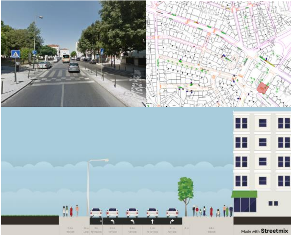
Figure 152. Cross-section of Praça Paiva Couceiro between Avenida Mouzinho da Silveira and Rua Morais Soares
