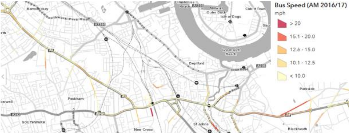
Figure 39. Bus speeds in the morning peak for the year 2016/17, showing westbound speeds mostly below 10mph
