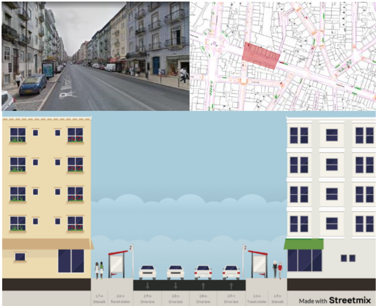
Figure 147. Cross-section of Rua Morais Soares between Rua Francisco Sanches and Rua Cavaleiro de Oliveira
