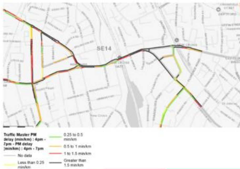
Figure 215. Data showing the level of delay experienced by vehicles, with darker colours showing greater levels of delay
