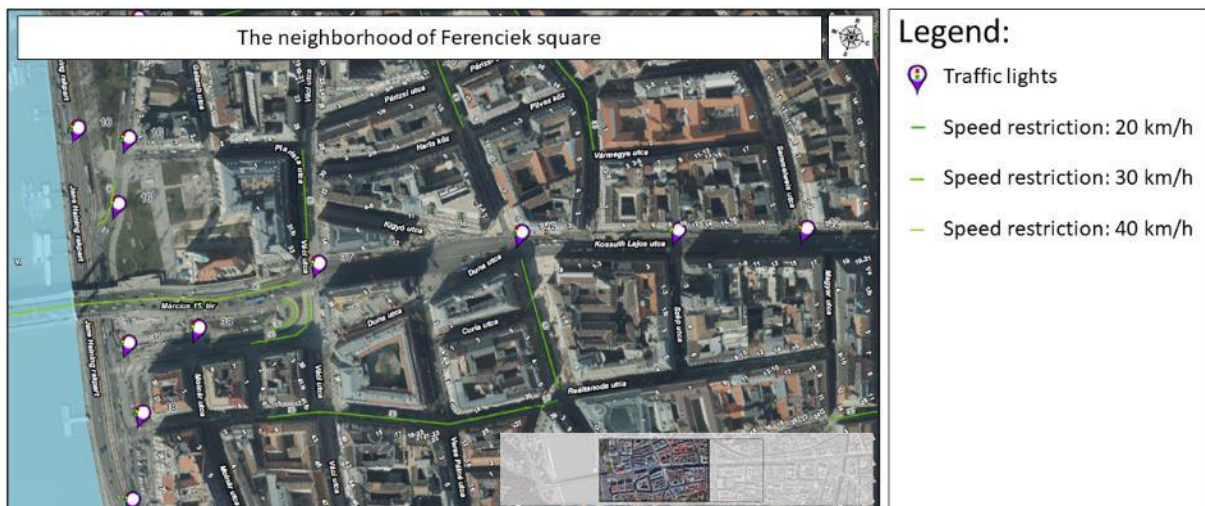
Figure 120. Traffic lights and speed restrictions around Ferenciek square (S8 Erzsébet bridge, I9 Ferenciek square, S9 Kossuth Lajos street)
