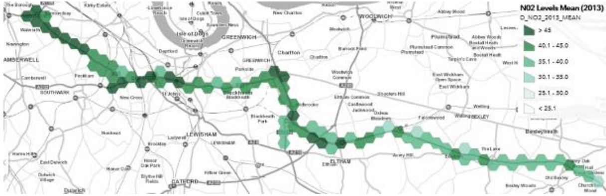
Figure 33. Modelled mean NO 2 concentrations (µg/m 3 ) along the A2 for the year 2013. Darker hex cell indicates higher concentrations
