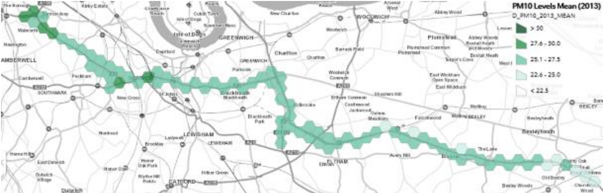
Figure 34. Modelled PM 10 concentrations (µg/m 3 ) along the A2 for the year 2013. Darker hex cell indicates higher concentrations
