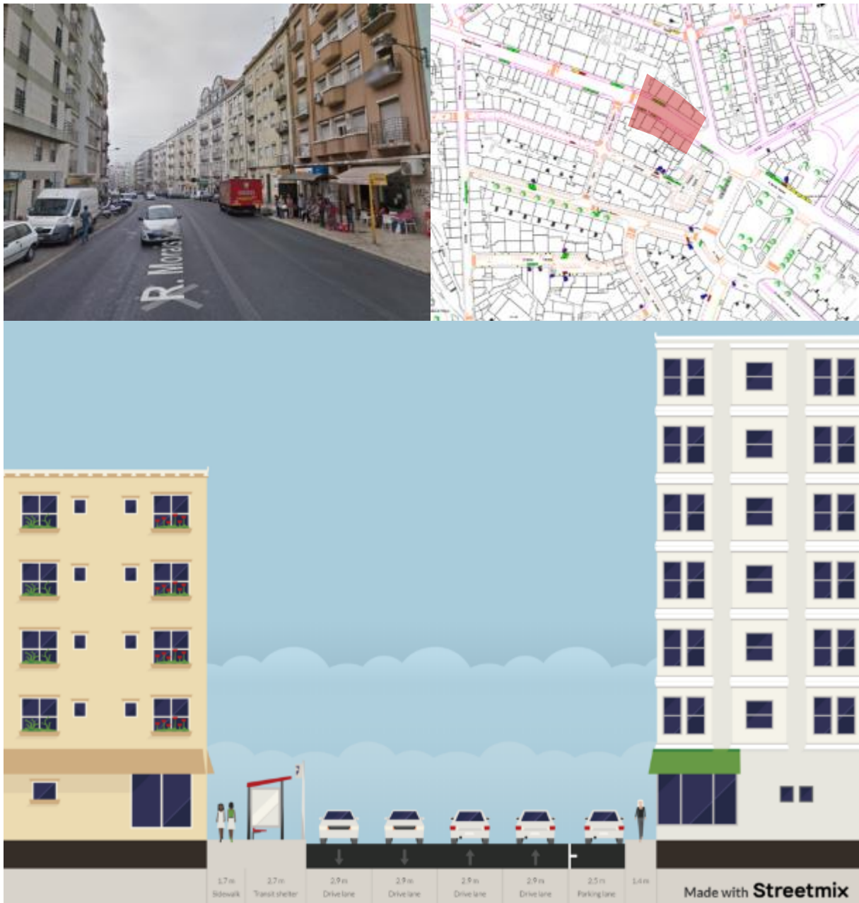
Figure 149. Cross-section of Rua Morais Soares between Rua Carrilho Videira and Rua Barão de Sabrosa
