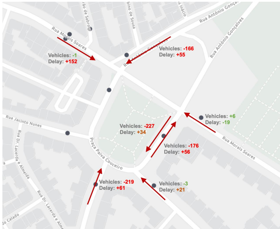
Figure 296. Difference of the number of vehicles and delay time between current scenario and suggested scenario for Praça Paiva Couceiro, AM Peak
