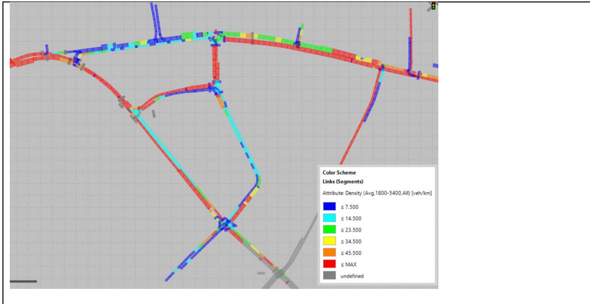
Figure 207. Model Comparisons (Current Situation v Public Transport Priority v Place Priority) Vehicle density Segment 2
