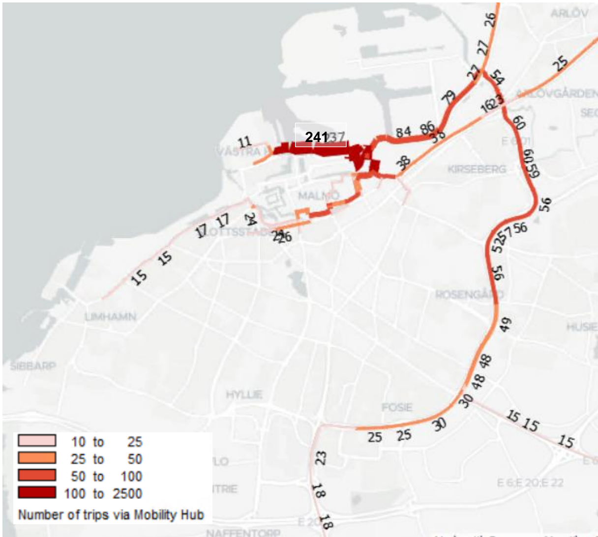
Figure 218. Number of trips via mobility hub travelling on each link (showing if more than 10). Morning peak hour parking fee 100 SEK per day.
