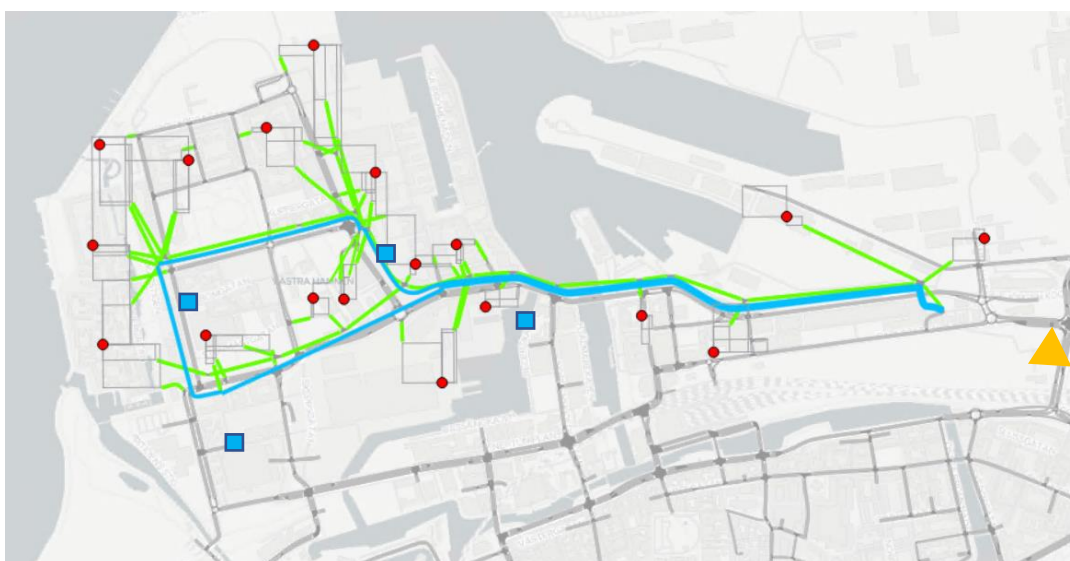
Figure 216. Implementation of shuttle bus (blue) and bike/electric scooter (green) paths between the mobility hub (orange triangle) and the destinations in the Western harbour and Nyhamnen area (red dots). The road network is represented in grey.
