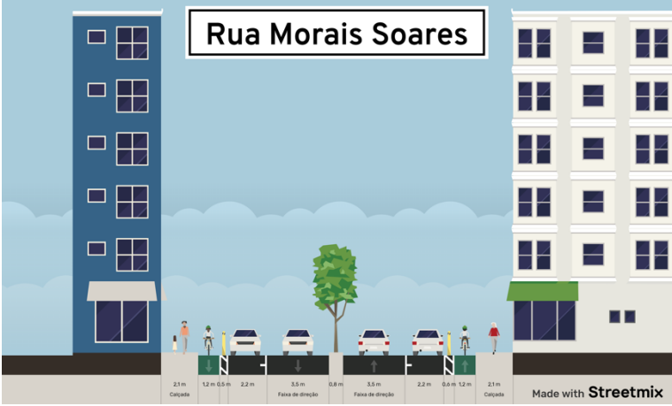
Figure 78. Suggestion 2: Reduction of one lane in each way, maintain existing parking and introduction of one cycle lane in each side of the road. Slight sidewalk enlargement.
