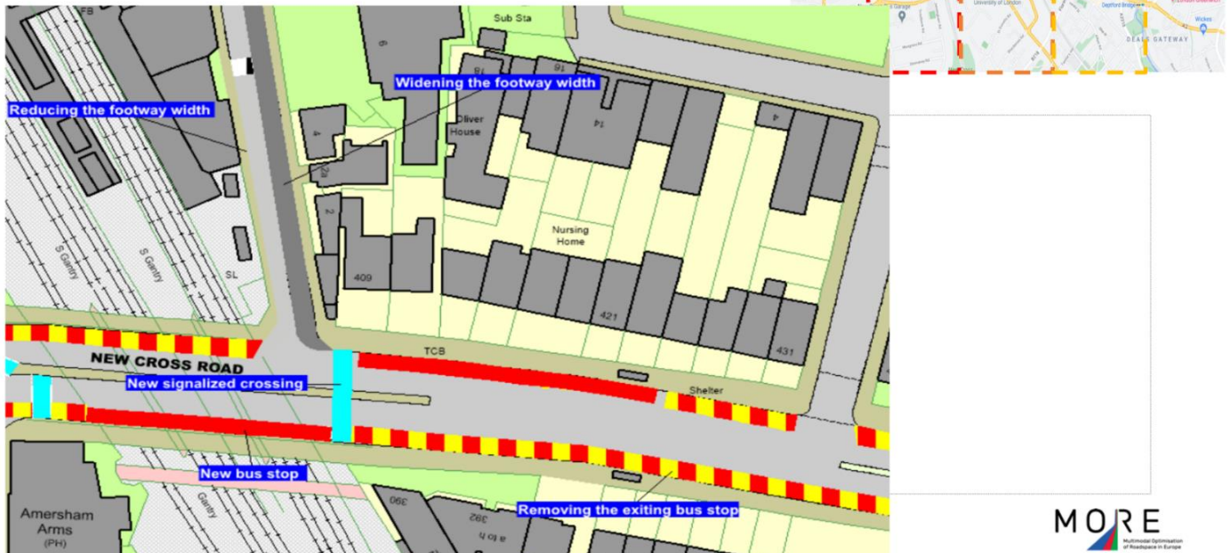
Figure 188. Annotated changes made to the East Segment of the Stress Section for Public Transport Priority design options
