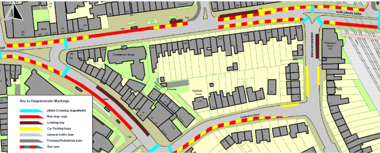
Figure 189. Annotated changes made to the Central Segment of the Stress Section for 1-way operation of the gyratory for Public Transport priority design options
