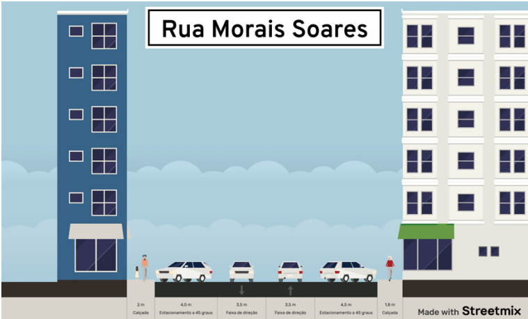
Figure 77. Suggestion 1: Reduce of one lane in each way and introducing of diagonal parking
