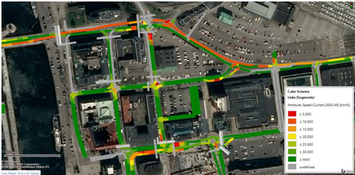
Figure 220. Morning rush hour without gating, the western part of the model, average speed
