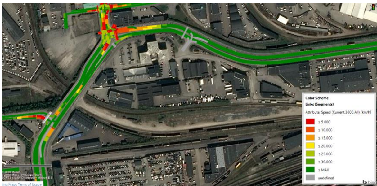
Figure 221. Morning rush hour without gating, the eastern part of the model, average speed
