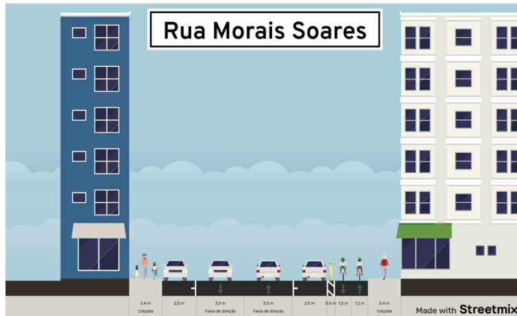
Figure 81. Suggestion 5: Removal of one lane each side and introduction of two-way cycle lane in one of the sides. Sidewalks are enlarged.
